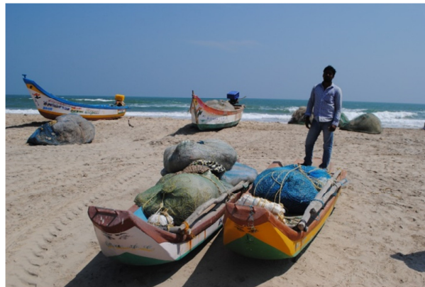
FRP Kattumaram of the East Coast. The craft is used by one or two persons for small time fishing
