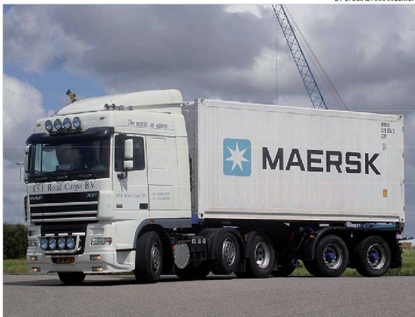
A container with ultra-deep freezer capable of maintaining temperatures of upto minus 60 degrees centigrade
